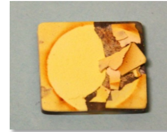
T1-5: Coupon tested in water vapor at ~1482°C (2700°F), 49, 1 hr cycles
