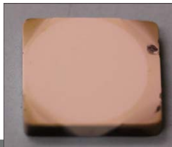
T2-5 Coupon tested in water vapor at ~1450°C, 50, 1 hr cycles
