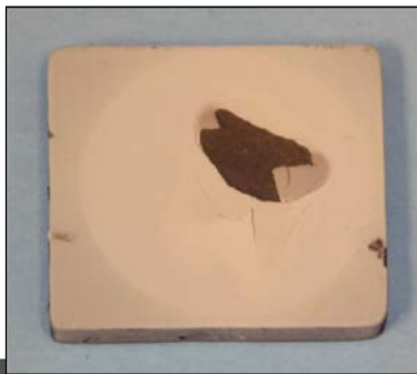
T2-4 Coupon tested in water vapor at ~1300°C, 20, 1 hr cycles
